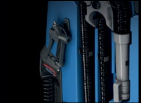
Sanitizing sprayer to sanitize the machine at the end of the shift (only available with the Disinfectant)
